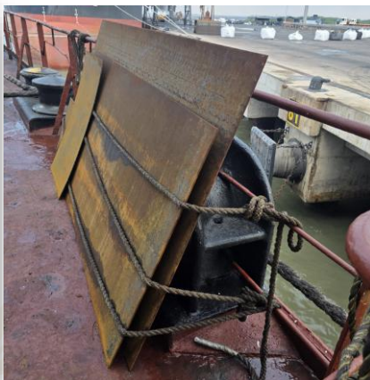
Mooring fair lead obstructed by heavy plates
