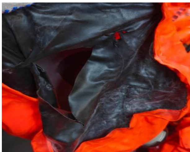
Badly damaged Engine room EEBD mask
