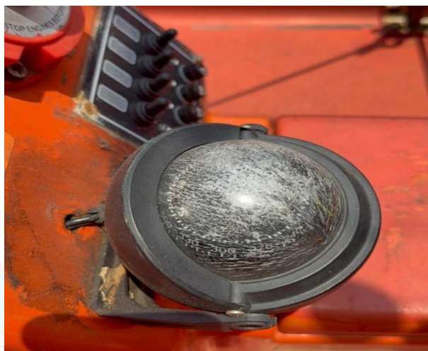
Rescue boat magnetic compass enclosure cover found foggy
