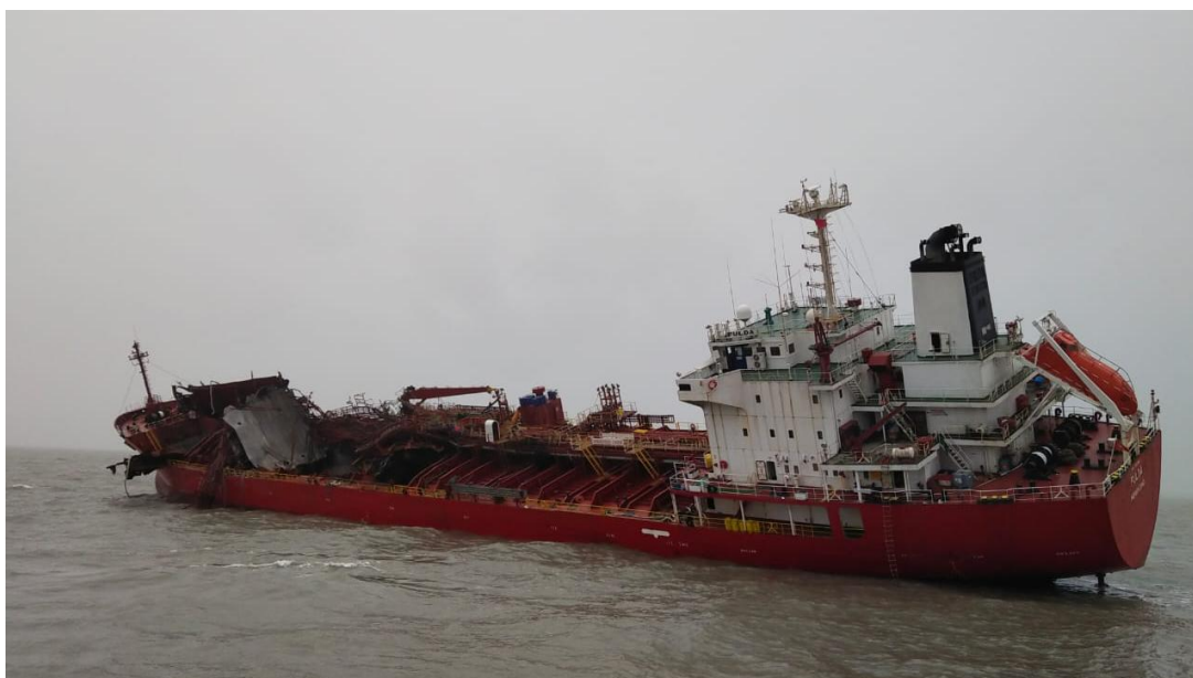
Figure 10 Fire and Explosion on MT FULDA
