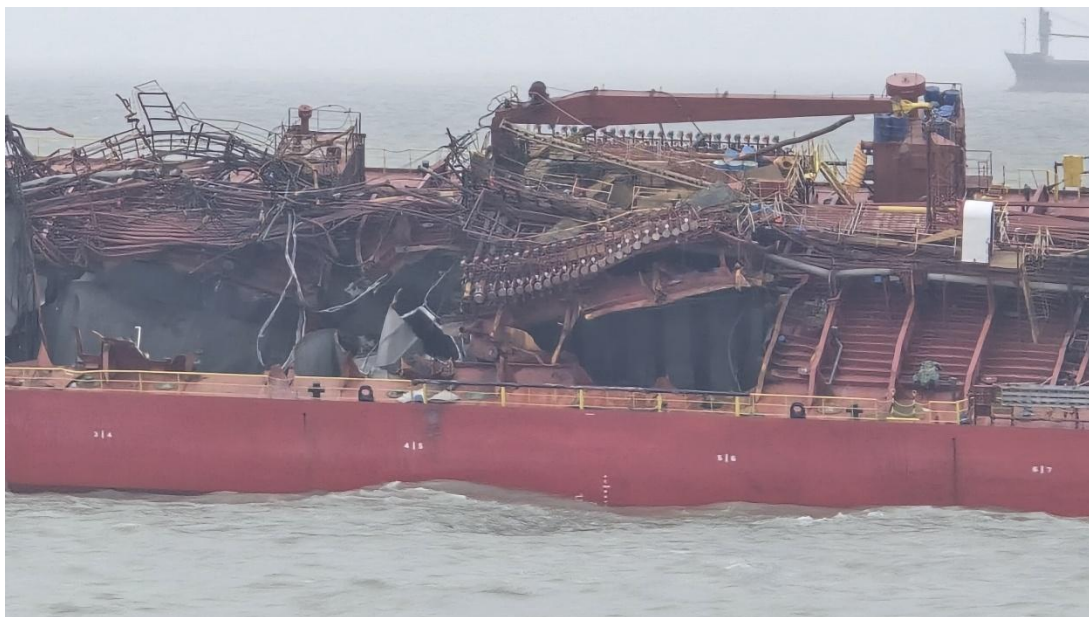
Figure 11 Fire and Explosion on MT FULDA
