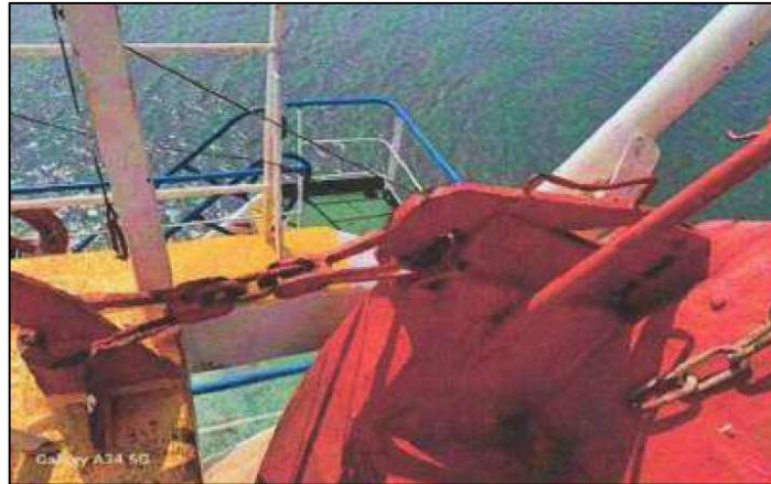
Figure 4: The FFLB in its stowed position on the launching arrangement, showing the securing arrangement.
