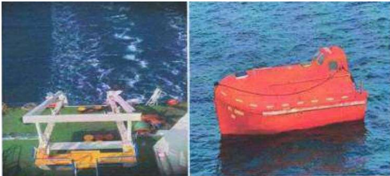
Figure 2: Stowage position of the FFLB. Left: the empty cradle after the release. Right: the FFLB as sighted in the water.
